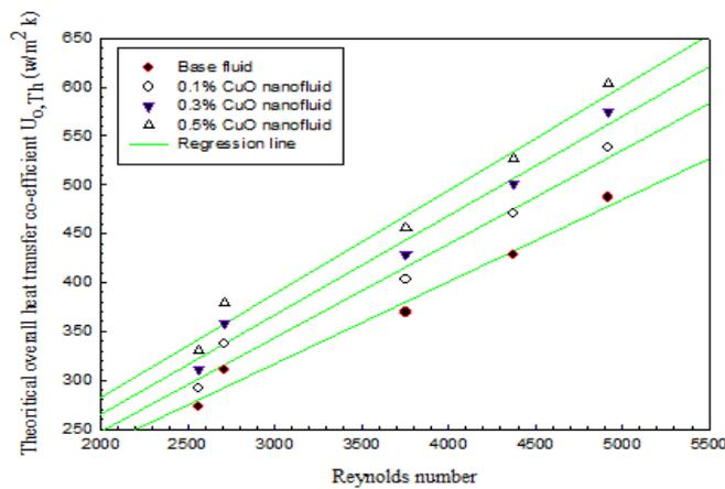
**Figure 5: Effect of Reynolds of CuO –Water Nanofluid on Theoretical Overall Heat Transfer Coefficient**
