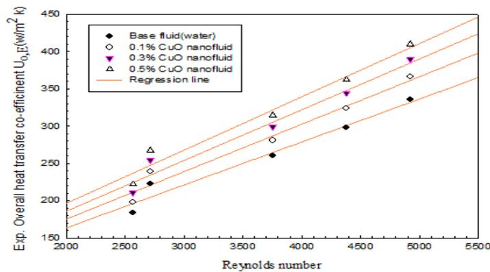
**Figure 4: Effect of Reynolds Number on Experimental Overall Heat Transfer Coefficient**
